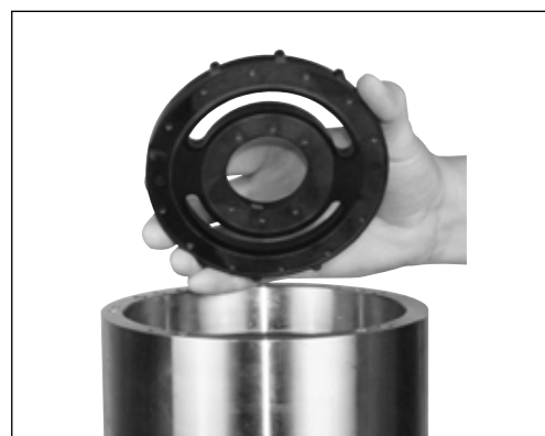
10. Mount port plate. Be aware of orientation/guide pin.
