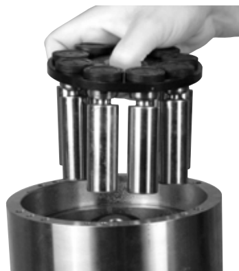
10. Remove pistons and retainer plate.
