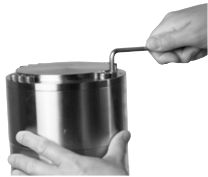
8. Loosen and remove 10 screws.
