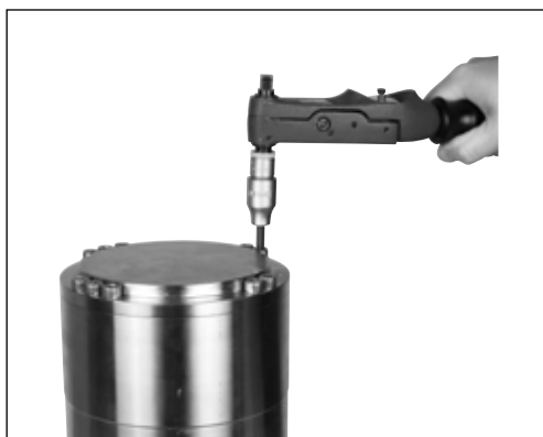
31. Tighten 10 screws to 30Nm.
